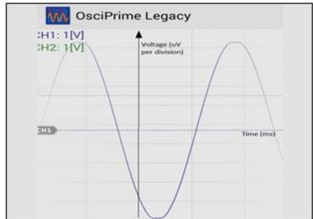
**Figure 2: The OsciPrime visualization of slight voltage clipping of microphone input at 100mV.**
