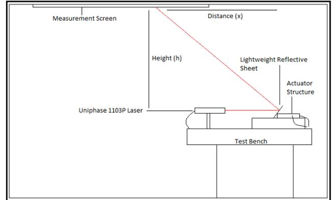
Figure 7: Diagram of the actuator test apparatus.
