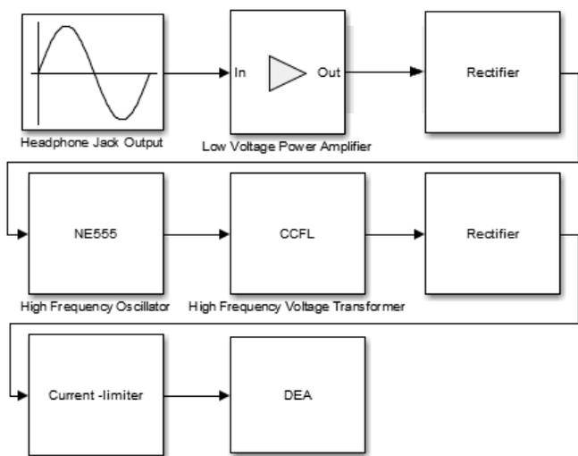
**Figure 4: Block diagram of stages between smartphone headphone jack output and input to dielectric actuators (DEAs). The headphone jack output is amplified and rectified to be used as an enable (activation) signal for a**
