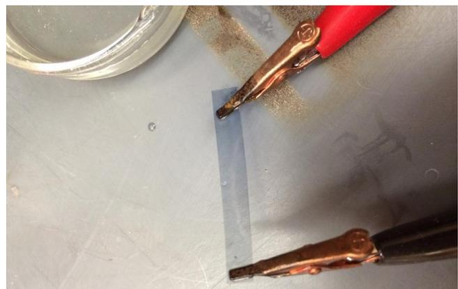
**Figure 5: Conductive PEDOT strip dipped in a Lithium perchlorate solution with an applied +5V on the upper clip. A reversible visible change in color can be seen.**
