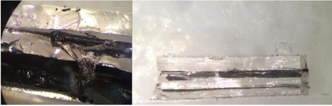
Figure 6: Dielectric breakdown of ~0.500mm Sylgard (on the left) and the DEA before testing.
