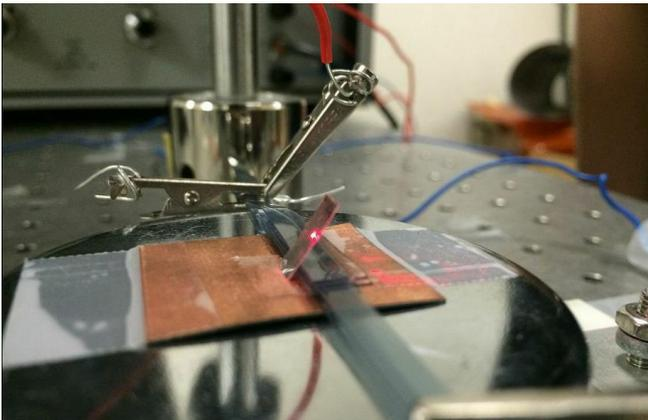
**Figure 8: Sylgard 184 and Conductive foil bi-layered stack.**
