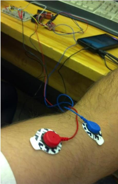
**Figure 1: Disposable adhesive silver/silver chloride EMG electrodes attached to the subject's bicep. The red and blue electrodes form the differential pair, as (to be discussed in Section 3.2). The third reference electrode is hidden. The image also shows connections between the electrodes and Muscle Sensor, Muscle Sensor and input attenuation circuit, and input and phone (also discussed in Section 3.2).**
